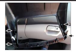
3. Remove 4 screws to disassemble OEM-Case from OEM-Panel
