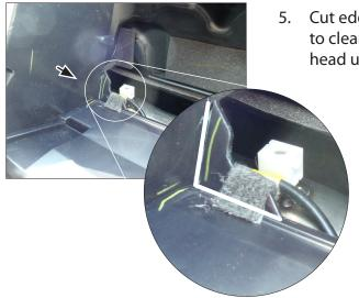
5. Cut edges at the left and right to clear space for Double-DIN head unit
