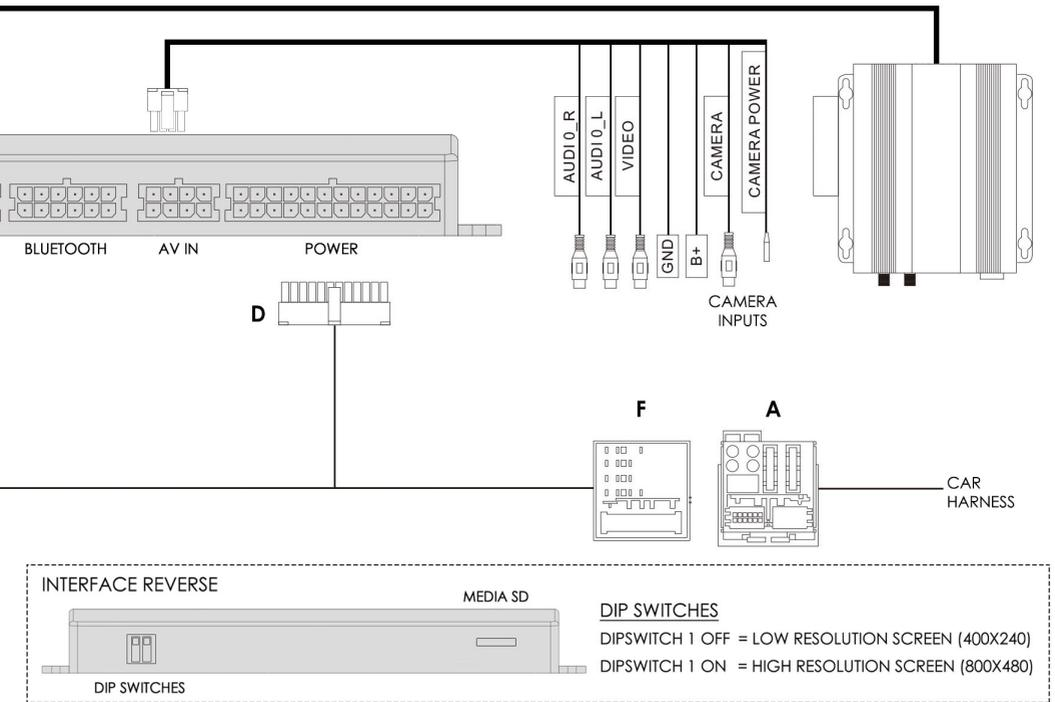
1. Remove the OEM head unit and disconnect the main power Quadlock (A).
