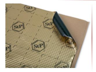
Multicomponent polymer based on butyl rubber supplemented with anticorrosive excipients. The material is a resinous construction of black color with the adhesive layer covered with corrugated aluminum foil of golden color with black printing and small cell stamping. The adhesive layer is covered with the
