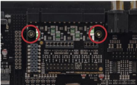
2. Pull the board upwards. Now you have access to the jumpers of the channels A to F (J 3 & J 4).
