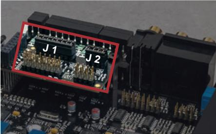
The jumpers of the channels A to F are located underneath the highlevel expansion board. To get access to the jumpers follow the subsequent steps:
