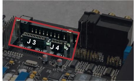
For repositioning a jumper simply pull it upwards and plug it to the desired plug position.
