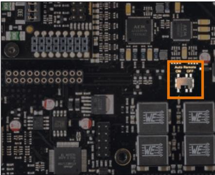
On: Activation via highlevel speaker input is enabled (ex works).
