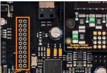
6. Make sure that the HEC module is installed properly and all pins are fully inserted into the socket.
