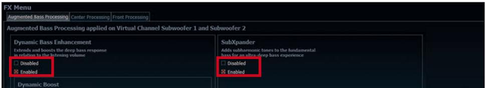
Note: the bass processing is switched on and off together for both “Subwoofer 1” and “Subwoofer 2” channels, nevertheless the two channels still remain separately processed for stereo applications.
