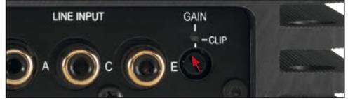
However, it is possible to optimally adapt the input sensitivity to the signal source using control 10 (*Gain*) and by repositioning jumpers inside the device (see page 28, item 4; Adjustment of the input sensitivity).
